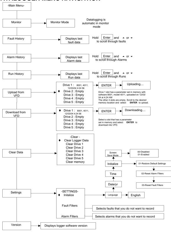
The Monitor Mode provides for Real-Time display of Inverter operation. It also indicates the total number of Run events, Alarm and Fault events.
