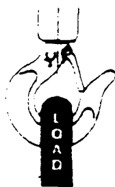
SEAT LOAD CORRECTLY IN HOOK
