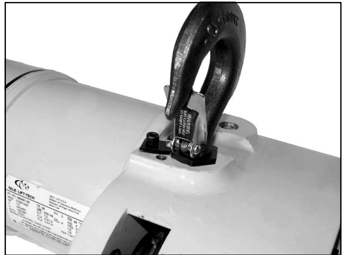
Figure 7-18. Removing Upper Hook and Hook Nut from Hoist Frame (1/4 thru 1 Ton Models)
