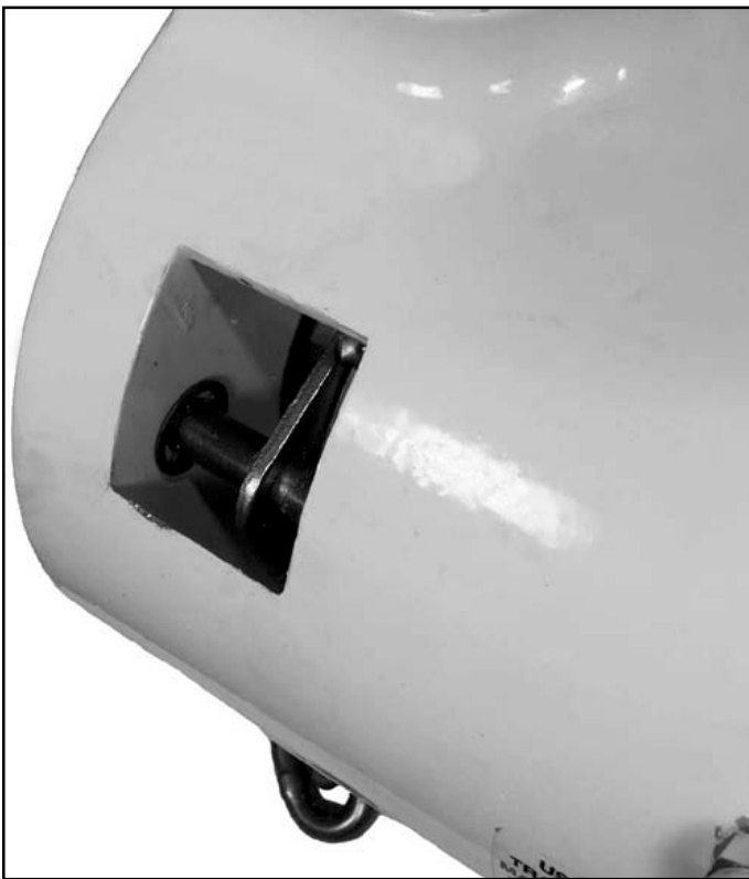
Figure 7-13. Removing Chain Guide Support Pins
