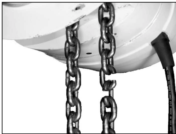
Figure 5-4. Installing Coil Load Chain Using Two "C" Links (1/4, 1/2 & 1 ton hoists)
