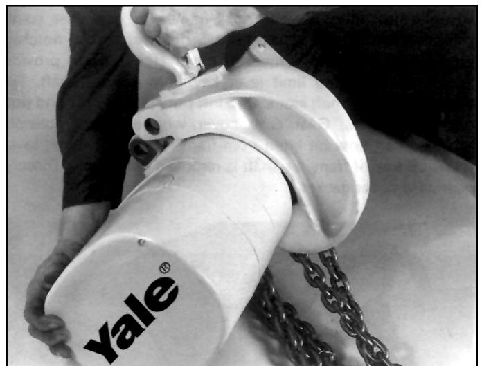
Figure 7-3. Removing 3 Ton Hanger Bracket from Hoist Frame
