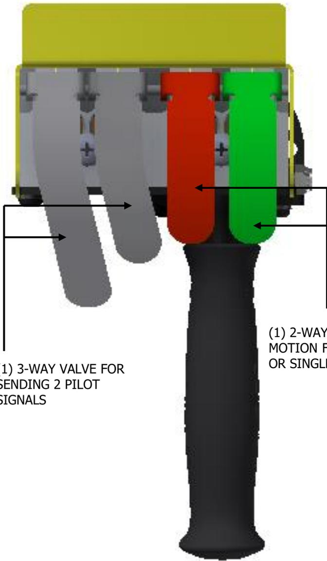
(1) 2-WAY VALVE FOR UP/DOWN MOTION FOR AN AIR BALANCER OR SINGLE ACTING CYLINDER
