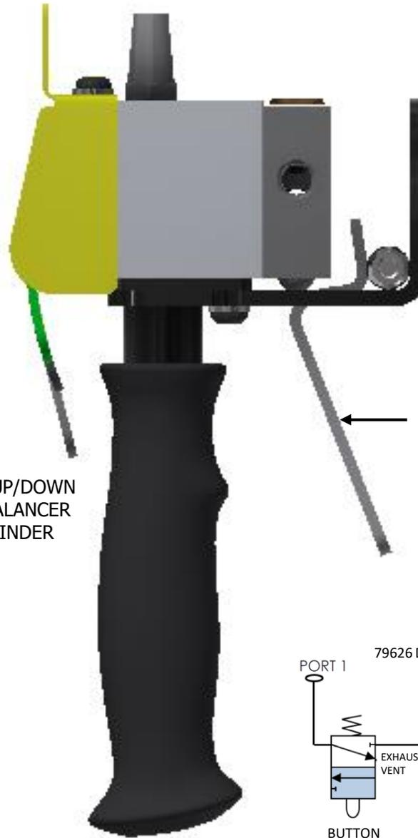
TRIGGER: 3-WAY VAL' USED FOR SENDING 1 PILOT SIGNAL
