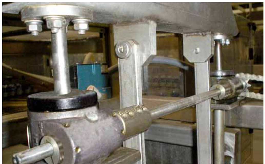
Shown are two of four M2555 Series 1/4 ton actuators.
