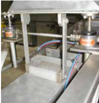
Two actuators shown in a four actuator system to adjust conveying system.
