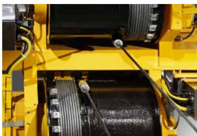
Off-standard rope drum for accommodating a work rope, with a recess for the fast action lock available as an option.
