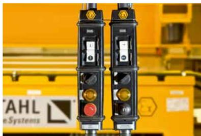
The SWH 5 ex control pendants are specifically designed for controlling hoists and cranes in hazardous areas. For explosion-proof wire rope hoists, the two-stage control unit SWH ex is used in protection type flameproof enclosure »db« and increased safety »eb«, as well as in IP66 and protection by enclosure »tb«.
