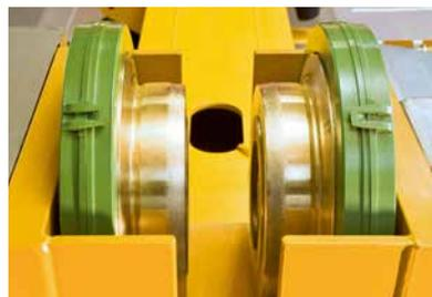
The protection type of all wheels is constructional safety »c«. Among other measures, wheels are made of brass for high travel speeds.
