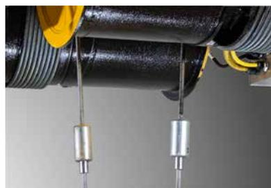
The client's off-standard ropes for pump maintenance are connected by rope locks. With the aid of the fast action lock, the hoist can easily be equipped with a bottom hook block to suit its application.
