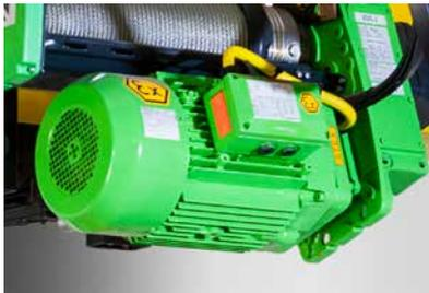
Motors for Zone 1 and Zone 21 are of grey cast iron, protection is a combination of flameproof enclosure »db«, increased safety »eb« and protection by enclosure »tb«. For Zone 2, the motors are made of aluminium and have the protection class increased safety »ec«. For Zone 22 the motors are in IP66 and with protection by enclosure »tc«.
